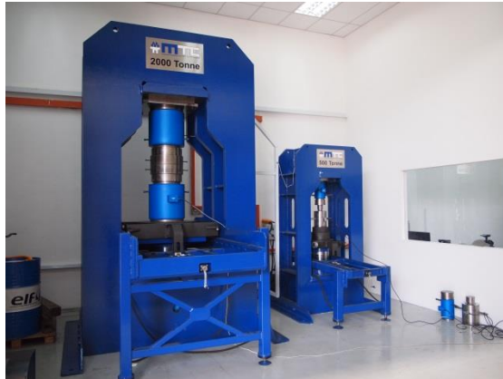
(Left) Singapore's first 20 MN force calibration facility
